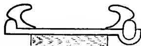
Cross Section, Michelin Quick Detachable Rim, with rings adaptable to clincher type tire
